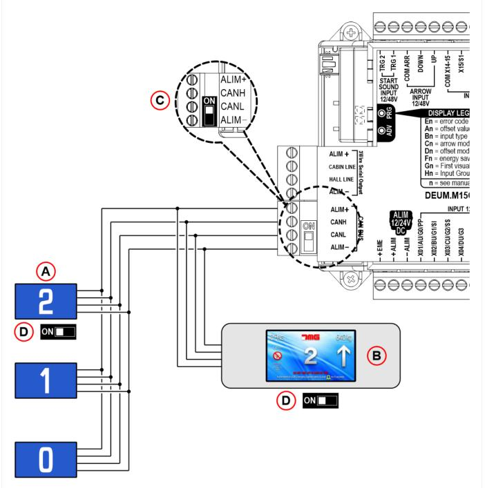
A) – CAN serial Position Indicator (Floor)
