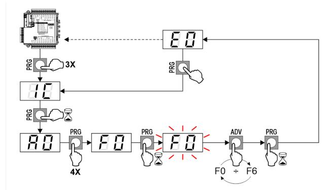
F0 (Default) = Disabled function: Supply the "S8" input (see "Indicators and emergency lamp inputs") to command the function from other unit.
